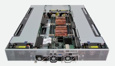
Figure 2. Cray CS-Storm 2U server containing up to 8 NVIDIA Tesla K80 GPUs used for running ECHELON.
