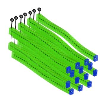
Figure 1. Plot of 14 horizontal multi-staged fractured wells. The fractures and the completions can be seen for all the wells.
